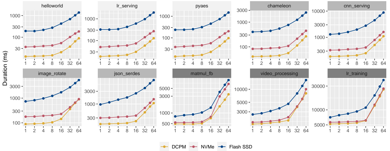
Figure 4: Average cold start latency as the number of microVMs restored from snapshots in parallel increases. (Note that vertical and horizontal scales are \log_{10} and \log_2 , respectively, with the former being different per function.)
