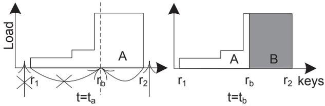
Fig. 8. Smart remote node placement: Node A scans its range and decides to place B on its forward direction, minimizing the number of transferred items  $|r_2 - r_b|$ .
