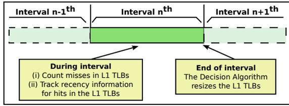
**Figure 5:** Lite divides the execution time of an application into *intervals*. During each interval, Lite tracks the performance of L1 TLBs. At the end of each interval, Lite decides whether to resize the L1 TLBs.
