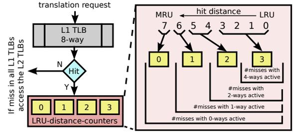
**Figure 6:** Lite introduces *lru-distance-counters* per L1 TLB to track the utility of ways [20, 46]. The corresponding counter is increased on each L1 TLB hit depending on the distance from the LRU position. At the interval end, each counter holds the number of L1 TLB misses that would have occurred, if those ways were disabled.
