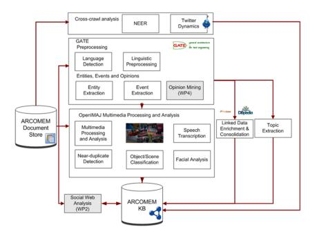
Fig. 1: Processing chain for ETOE extraction, analysis and enrichment
