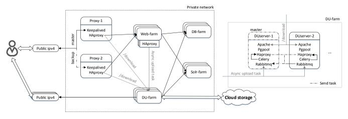
Fig. 3: Data storage and serving: DU-farm architecture and integration
