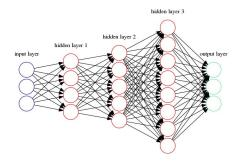
Fig. 2: Example of a three hidden layer neural network
