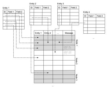
Fig. 2: Event Log and Entites storage using star schema.
