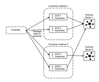
Fig. 4: Connectors inside the BDA
