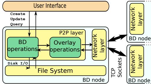
**Figure 3: Architecture of a BD network node**
