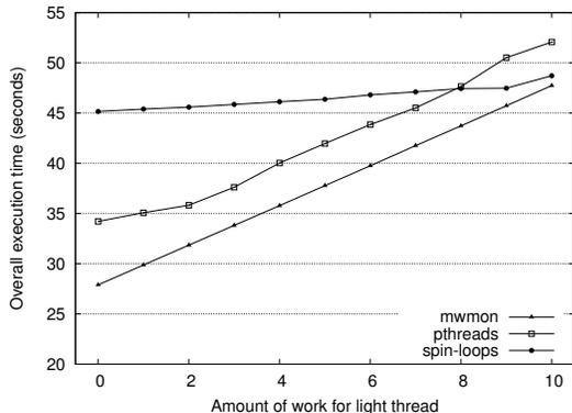
**Figure 4. Throughput of various barrier implementations for different levels of threads asymmetry (see Fig. 3b).**
