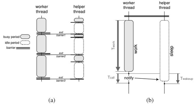
**Figure 2. (a) Application model under consideration. (b) Execution scenario for the evaluation of condition-wait and notification primitives.**
