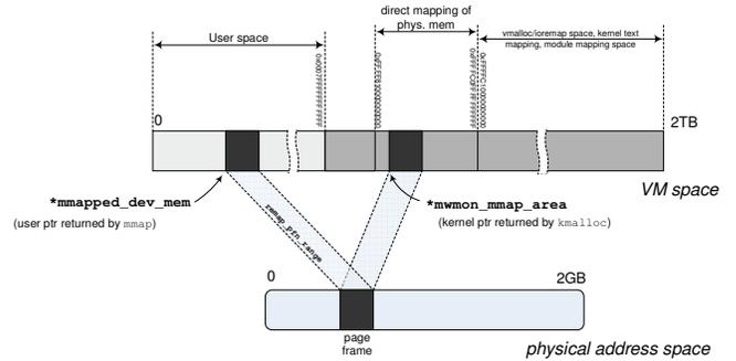
**Figure 1. Mapping the monitored memory region allocated at kernel-space to process address space.**
