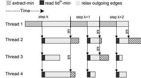
Fig. 3: Execution pattern of the HT scheme.
